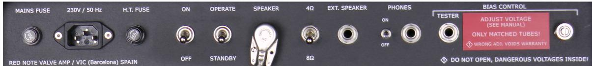
**Main Fuse** - This fuse protects the power transformer primary and the value is 3A/250V Slow- Blown type. Please it is very important to change the fuse with the same type and value. Failing to do that will invalidate the warranty
